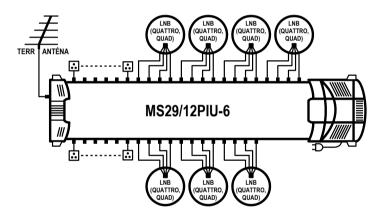
Connection of multiswitch for satellite reception from 8 satellites and distribution of terrestrial signals:
