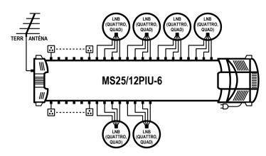
Connection of multiswitch for satellite reception from 7 satellites and distribution of terrestrial signals:
